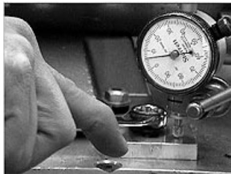
3. A precision soft foot check should be completed before and after precision alignment has been performed.
