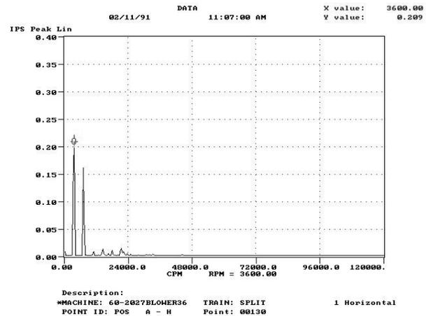
As with any analysis process, when using vibration analysis to detect misalignment care should be taken to gather and analyze a sufficient amount of data, including spectral data, amplitude data, phase data, and time waveform data. It should also be noted that all misalignment problems do not reveal the clear symptoms listed above. Some misaligned machines simply do not react vibration-wise according to these textbook symptoms.
