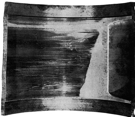
In plane or sleeve type bearings, misalignment often results in either an angular wear track of a pattern referred to as "cross-corning."
